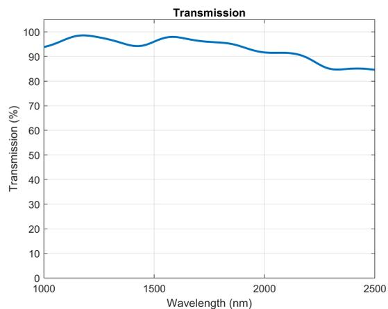
Figure 6. Transmission as a function of wavelength (lens only). Measured data is scaled with respect to the F-numbers ratio.
